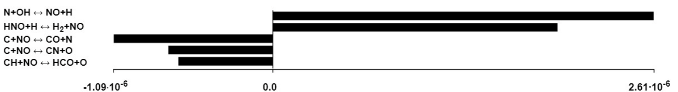
Figure 10. NO formation rate for set of reactions implemented for calculations.
