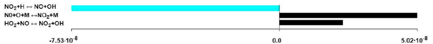
Figure 12. \text{NO}_2 formation rate for set of reactions implemented in calculations.
