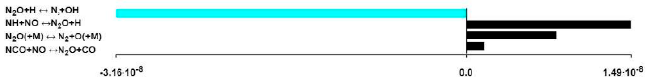
Figure 11. N_2O formation rate for set of reactions implemented for calculations.
