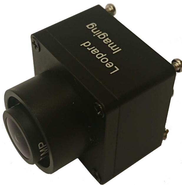
Rys. 6.11. Kamera Leopard Imaging LI-USB30-IMX390-GW5400-GMSL2-120H.
